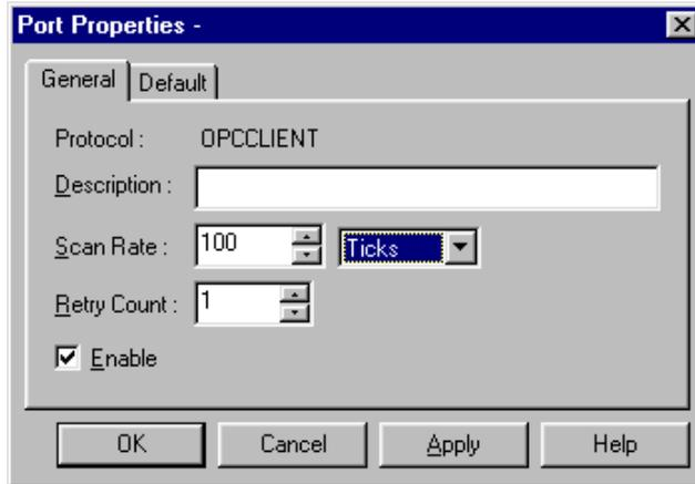
Scan rates are handled a bit differently in Cimplicity 5.0. Cimplicity 5.0 now uses an INI file for each port that allows you to establish the rate at which data is scanned
