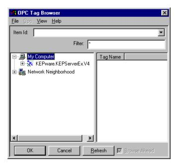
6. In the OPC Tag Browser tree view expand KEPware.KEPServerEx.V4 and then select Device\_1 under Channel\_1. A list of the tags available under Device\_1 will appear in the right-hand pane of the browser.
