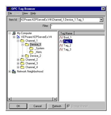
The Item ID for the Tag is KEPware.KEPServerEx.V4\Channel\_1.Device\_1.Tag\_1. If you had browsed to another PC in the network to select the tag the PC name would be included in the Item ID as follows \Remote\_Station\KEPware.KEPServerEx.V4\Channel\_1.Device\_1.Tag\_1.
