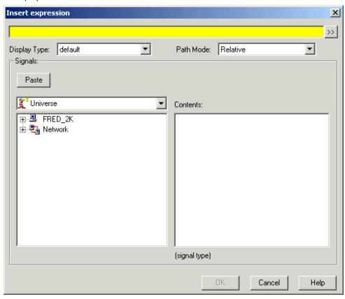
In the Signals section of the Insert Expression dialog you are going to expand the Objects in the left hand pane until you can see the folders under the OPCClient Object that you created. These folders are the Channels and Devices that were created in the KepserverEx project.
