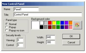
Click OK to accept the changes that were made to the panel and create it as an object in the process.
