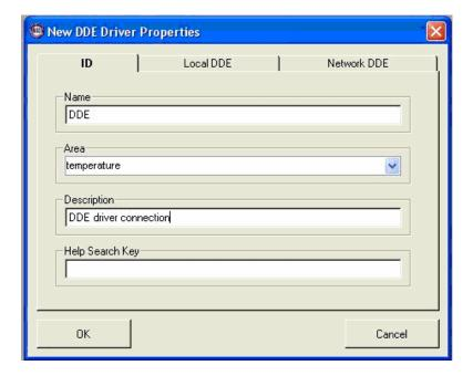
The **Driver ID** section is now complete. Click the **Local DDE** tab. In the **DDE Application Name** box enter the service name for the KepserverEx. The default name is **kepdde**, (this information can be found in the server Tools->Options->DDE tab in the **service name** text box). Enter the **DDE Topic Name** "\_**ddedata**". Click OK to finish the driver setup.
