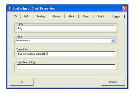
Click the **I/O** tab. The **I/O Device** text box should read, "No Tag Selected." Click the "..." button to the right of the text box to browse for the I/O Device. Select the OPC device created earlier by double clicking the name, or by highlighting the name and clicking the **select** button located in the bottom right of the window. In the **Address** text box, enter the address of the tag located in the KepserverEx. This should be entered in the following format:
