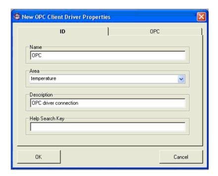
The **Driver ID** section is now complete. Click the **OPC** tab. In the **Automation DLL Prog ID** text box enter "**opc.automation**". In the **Server Prog ID** field enter,
