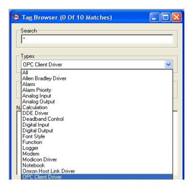
KepserverEx is capable of being an OPC or DDE server to VTS. If you define an OPCClient object in Lookout, then KepserverEx will be an OPC server to it.
