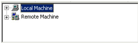
*LinkMaster uses OPCEnum for browsing and connecting to servers. If you cannot find a server but know that it is there it is possible that it is not properly registered as an OPC 1.0 or 2.0 server and you are using an older version of LinkMaster. Upgrading to the newest version of LinkMaster should correct this problem.*
