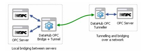
Can also be used with Tunnel/Mirror feature to bridge between data on network connected servers.
